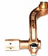
11296S Stewart Speedometer Drive Mounting Set (1923-1927)
