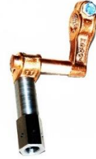
3986BS Stewart Speedometer Drive Mounting Set (1920-1923)
